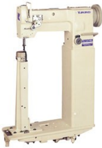
TK-1247HBL 1NEEDLE, LEFT-SIDE HOOK
