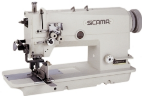
Needle Gauge: 9.5mm or 12.7mm Single welt or Double welt
